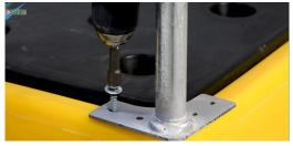
**b.** Loosen the grub screws on the angle brackets with a 6mm hex key and slide all four of the angle brackets on top of the vertical support bars.
