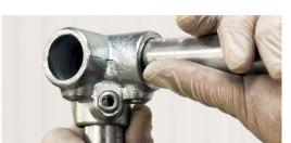
**d.** Push the remaining two bars in to the angle brackets. Ensure all are squared up and tighten the grub screws.
