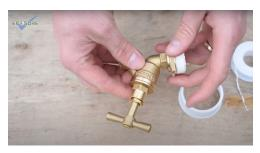
**d.** Screw the complete tap kit into the threaded outlet of your tank.
