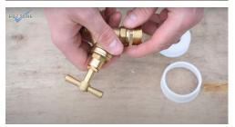
**c.** Wrap PTFE tap around the thread of the reducer.
