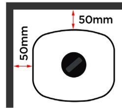
**a.** Tanks must be sited on a flat, level concrete base. If you are installing two water butts they must be level with each other.
