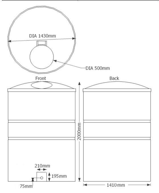
In order to allow us to meet the requirements of your order, please mark full details of all the additional connections you require on the diagram, stating sizes, distance from the edges, etc, and labelling the connections.
